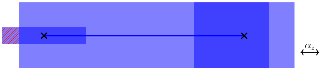
Figure 4.10: The minimum adjacent edge length rule, introduced in Section 2 on page 6 can be checked by considering each pair of adjacent edges of the polygonal boundary. There is a violation if there is a pair \{e, f\} such that both edges have length less than the threshold value \alpha_z . Its error-rectangle is the bounding box of e and f . Since the polygonal boundary is available checking this rule requires O(p) time. In this example, there are two violations involving the three short edges on the left. Both have the same error-rectangle, that is hatched in red.
