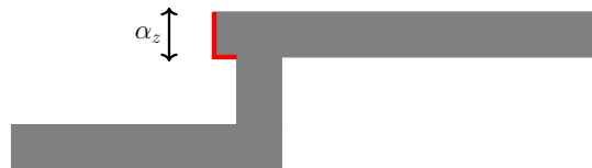
Figure 2.3: The gray shapes violate a minimum adjacent edge length rule of \alpha_z because of the two edges marked in red.
