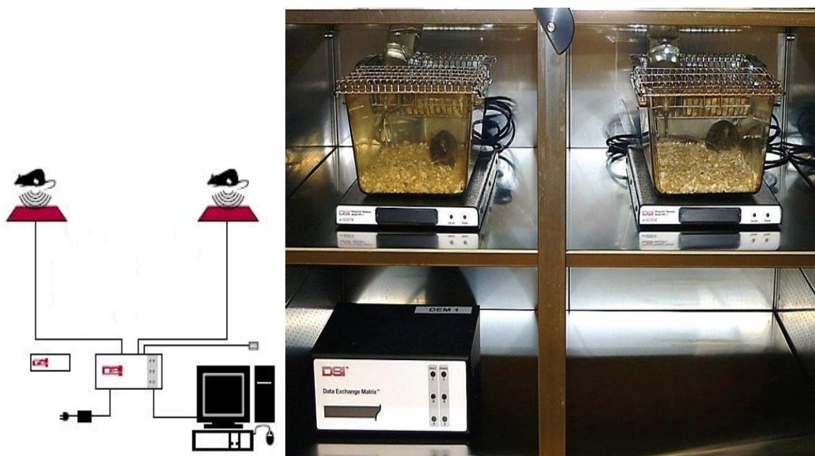
Figure 3.4: Each cage with an implanted mouse was placed on a receiver plate that was connected to a data exchange matrix. The EEG recording data was transferred through the receiver to the data exchange matrix and stored to the connected a computer.
