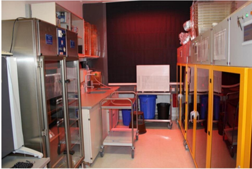
Figure 3.1: Ventilated cabinets for standard housing conditions for pre- and post-surgery placement and EEG recordings (Lundt, Wormuth, Siwek, Muller, et al., 2016; Papazoglou, Soos, et al., 2016).
