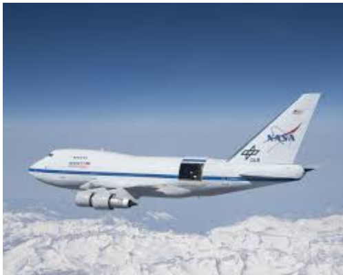
Figure 2.7: SOFIA soaring over the snow-covered Sierra Nevada mountains with its telescope door open during a test flight. Credits: NASA/Jim Ross.
