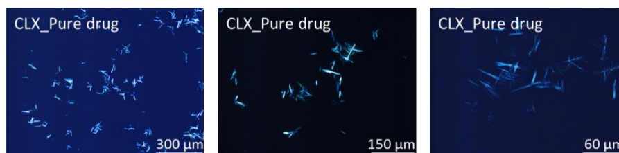
Figure 5.34: Micrographs obtained by PLM in a transmitted light modus at different magnifications (100x, 200x and 500x, respectively). The precipitation of pure CLX as needle-shaped microcrystals was confirmed.
