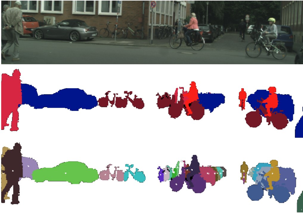
Figure 5.1: Desired workflow. Top: Input RGB image. Middle: Semantic segmentation mask. Bottom: Instance segmentation mask.
