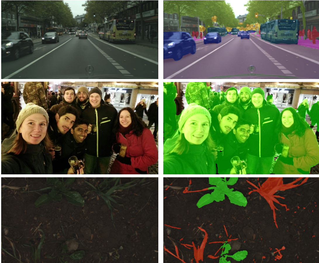
Figure 9.1: Sample predictions from Bonnet. Left: Raw RGB images. Right: Overlay with semantic segmentation label from CNN prediction. From top to bottom: Cityscapes dataset [30], person segmentation inferring a photo from our research group, trained on COCO [91], Crop-Weed agricultural dataset [22]. Best viewed in color.
