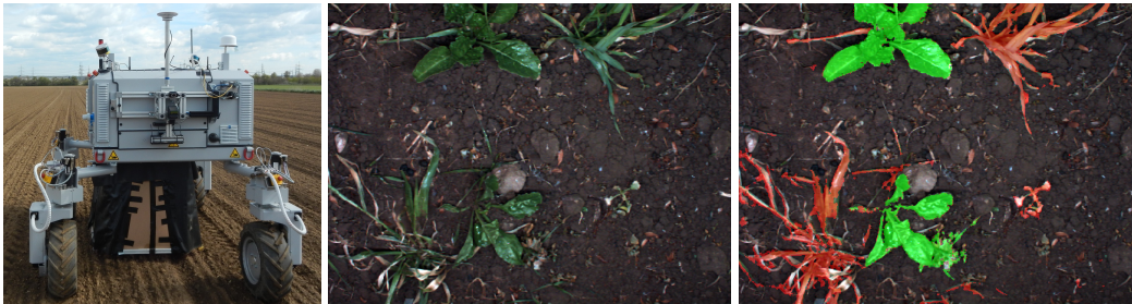
Figure 4.2: Left: BoniRob system, used for data acquisition and field deployment. Middle: RGB image captured during field test. Right: our corresponding classification result with crops colored green and weeds colored red.
