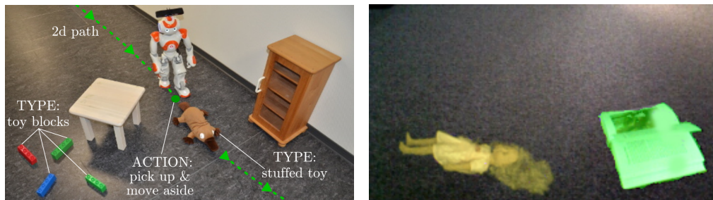
Figure 10.2: Room parsing for efficient path planning in children-inhabited environments. Left: Humanoid robot using information from semantics to plan. Right: Camera view with semantic overlay of different toys in the scene from Bonnet.
