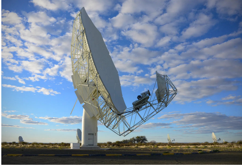
Figure 2.2: A MeerKAT dish. Between the main (big) reflector and the sub-reflector is the rotatable receiver platform. Credit: idia.ac.za
