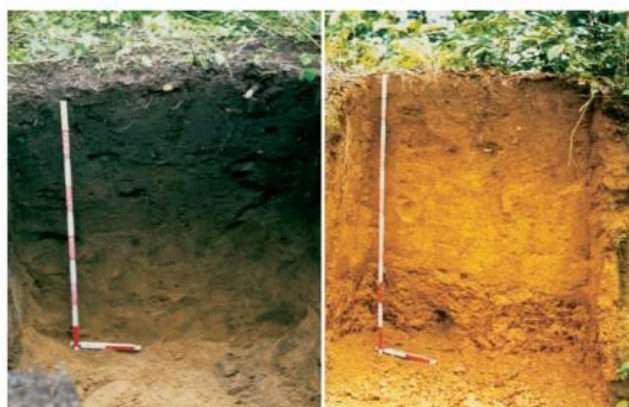
Figure 1.16. Typical soil profile of Terra Preta sites (left) and surrounding Ferralsol regions (right; Glaser et al. 2001).
