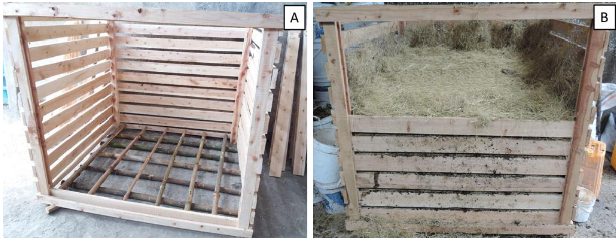
Figure A.6. Compost box. (A) Wooden compost box used for the composting trials, (B) Compost box filled with compost material (day 0) and with a layer of 10–15 cm teff straw placed on the bottom, back, front, left, and right side for insulation purpose.
