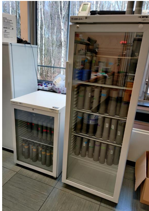
Figure C.1. Incubator with soil samples (280 PVC tubes).
