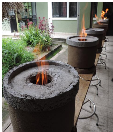
Figure A.2. Operation of the top-lit up-draft micro-gasifier (Noah stove; photos by Daniela Castro Herrera).
