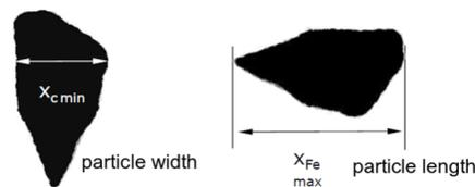
Figure 4.1 Two main particle size parameters analyzed with Particle Analyzer CamSizer: particle width ( $x_{cmin}$ , the shortest chord diameter), particle length ( $x_{Femax}$ , the longest Feret diameter) (adapted from (Microtrac Retsch GmbH, n.d.))
