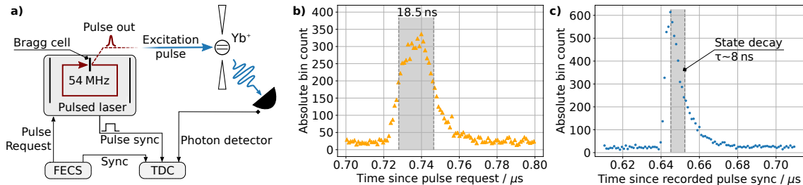
Figure 6.9: a) Sketch of the experimental setup used for synchronisation of the photon detection time stamps to the pulsed laser round trip frequency. The internal cavity of the pulsed laser is sketched as two mirrors confining the locked modes. b) Recorded time stamps of \sim 3,000 photon detection events extracted through the fibre cavity (to suppress pulse stray light). The detection timestamps are binned without a correction applied. c) Same data as in b) using the extraction times of the excitation pulses timestamp-wise as an offset for the photon detection timestamps. The x -axis of a) and b) shows the same scale to enable a comparison. The bin width is 1 ns.
