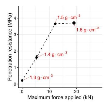
**Fig. 5.1** - **Resistance to root penetration**. Relationship between the maximum force applied by the testing machine and the penetration resistance measured by a hand penetrometer at different soil bulk densities. The soil densities is indicated in red. Each dot is the mean value among 12 data points. Error bars are the standard error of the mean for both axes.
