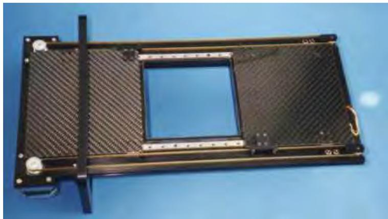
**Figure 2.4:** View of the Bonn Shutter before installing into BUSCA. The two black carbon blades are moved into the open state for testing.
