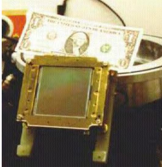
**Figure 2.6:** This figure shows one of the 3 “thick” CCDs in comparison to a one dollar bill just before mounting the device into one of the dewars.
