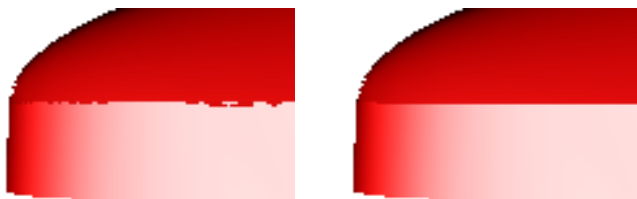
Fig. 4.12: Left: Aliasing artifact due to partly intersecting fat borders. Right: Pushing back the fat borders reduces the artifact.
