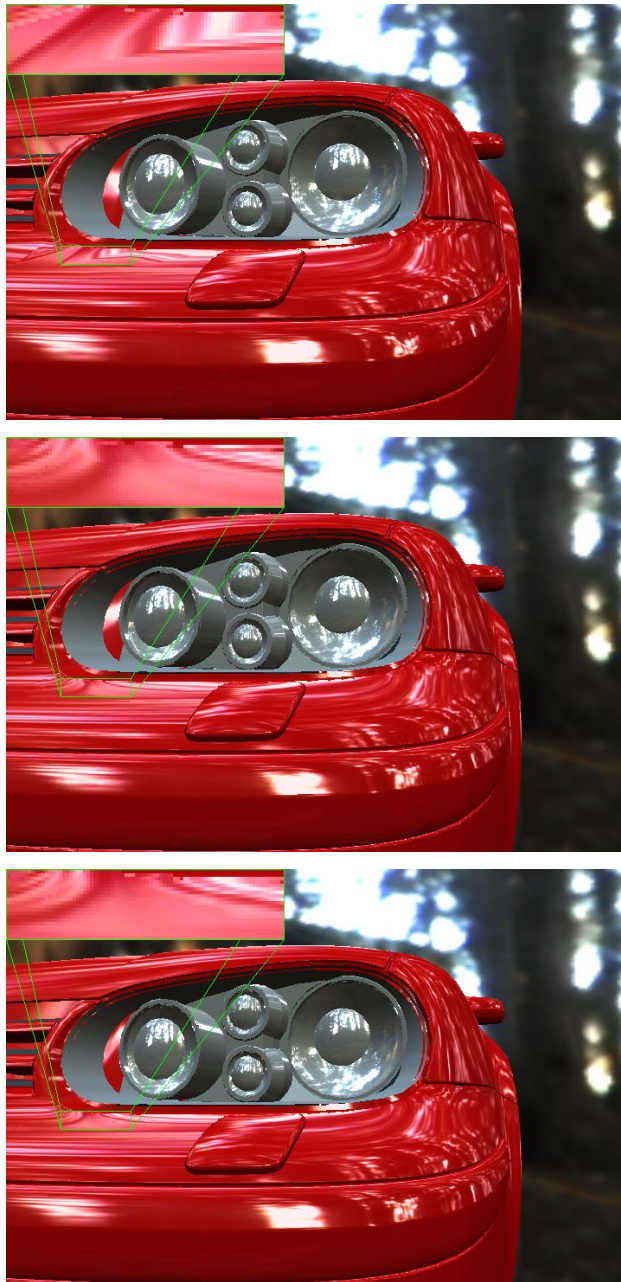
Fig. 9.8: A frame from the golf video sequence showing the results of standard tessellation (top), normal maps (middle) and appearance preserving tessellation (bottom).
