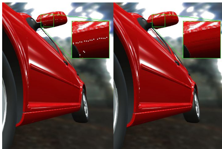
Fig. 4.16: View-dependent rendering of a car model without fat borders (left) and with fat borders (right).
