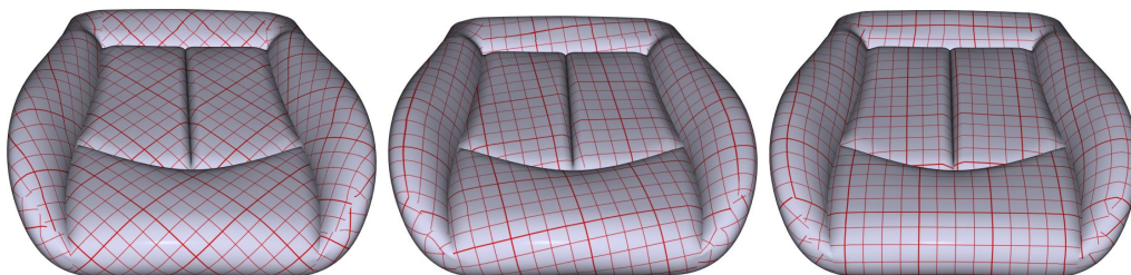
Fig. 7.3: Effects of different alignment strictness (from left to right: without, weak and strong rotation restriction)
