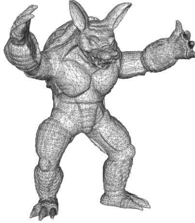
Figure 6.4: The Armadillo model, originally containing 345 944 triangles, simplified to 33 780 triangles.
