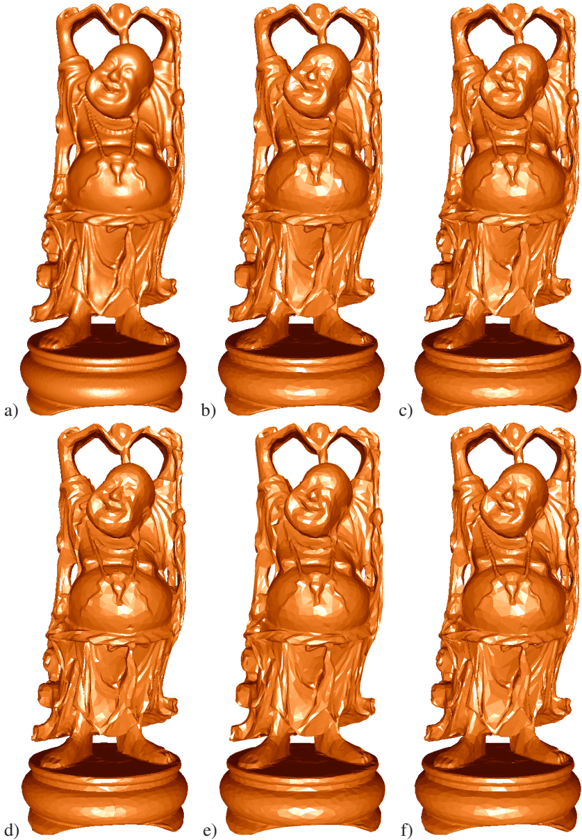
Figure 6.7: Results of applying different simplification methods to the Happy Buddha model: a) original model (1 087 716 triangles); b) QSlim 2.0 (18 338 triangles); c) OOCC (18 338 triangles); d) OEMM-QEM (18 338 triangles); e) stream decimation (18 486 triangles); f) our method (18 248 triangles).
