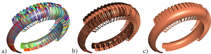
Figure 3.10: Model with 1250 patches: a) original model with patches shown in different colours and lighted from both sides; many patches overlap or are coplanar with each other; b) after applying our algorithm, several patches are still oriented incorrectly; c) the same model lighted from both sides.
