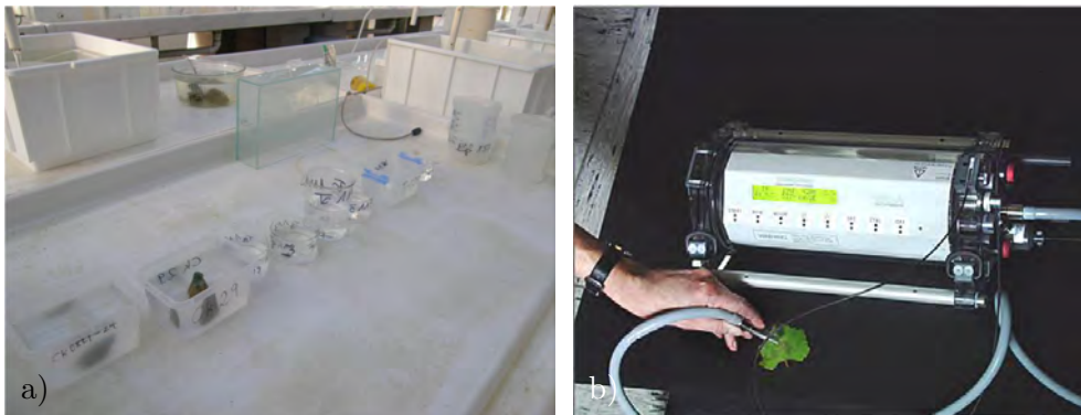
Figure 2.2 Measurements with a Diving PAM. a) Animals are kept separated from their food algae right after capture. b) PAM instrument. Photo: Heike Wägele.
