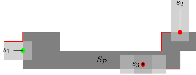
Figure 2.17: A pin \mathcal{P} with a set S_{\mathcal{P}} of shapes (dark gray), two wire stick figures s_1 , s_2 , and one via stick figure s_3 accessing \mathcal{P} , each creating a minimum edge rule violation. The violations caused by s_2 and s_3 we want to avoid by computing access areas which do not contain the corresponding access points (red dots). The violation caused by s_1 , however, depends on the length of l(s_1) , therefore the green access point will remain in our access areas unless other kinds of errors can occur.
