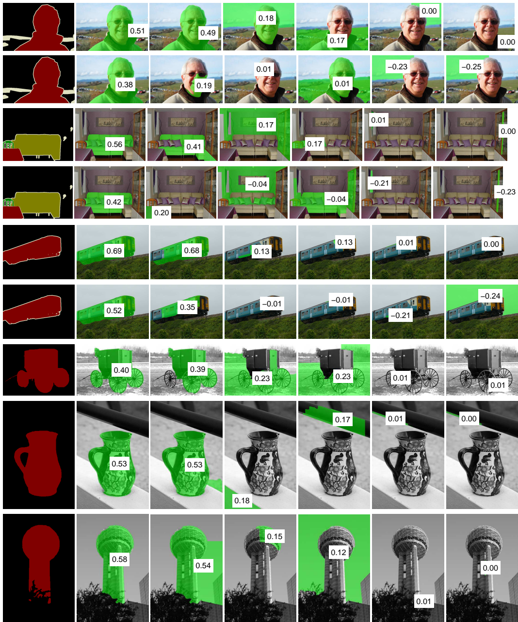
Figure 2.6.: Segmentation and ranking results obtained using the random forests model learned on the VOC2009 training set, with the features described in sec. §2.4. The green regions are the segment foreground hypotheses. The first image on each row shows the ground truth, the second and third images show the most plausible segments given by CPMC, the last two images show the least plausible segments, and the fourth and fifth images show segments intermediately placed in the ranking. The predicted segment scores are overlaid. The first three images are from the VOC2009 validation set and rows 2, 4 and 6 show the diversified rankings, with \theta = 0.75 . Note that in the diversified ranking, segments scored nearby tend to be more dissimilar. The last three rows show results from the Weizmann Segmentation Database. The algorithm has no prior knowledge of the object classes, but on this dataset, it still shows a remarkable preference for segments with large spatial overlap with the imaged objects, yet there are neither chariots nor vases in the training set, for example. The lowest ranked object hypotheses are usually quite small reflecting perhaps the image statistics in the VOC2009 training set.
