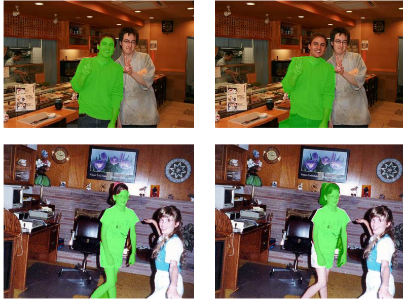
Figure 1.2.: Illustration of issues involved in segment ranking. After bottom-up segmentation (here using CPMC), recognition can be posed as selection among multiple sampled segments and a set of labels. While there are usually multiple segments covering each object, segments that align perfectly with objects may not always, if ever, be sampled. What seems important is to select the segment that best covers each object. Secondly, the ranking is affected by occlusion. In the images above, the segment covering the upper body of the girl is undesirable since there is a better one covering her full body. In the other image the segment covering the upper-body of the man is the most desirable. These properties justify our ranking formulation to learning: segments are regressed on the predicted overlap they have with ground truth objects. This formulation encourages finer segment selection than standard learning approaches based on binary classification and handles better the part-whole issues. The segment covering the girl’s upper-body is not a negative example in our formulation, it is a ‘positive example’ which is learned to be ranked proportionally lower than the segment covering the full body.
