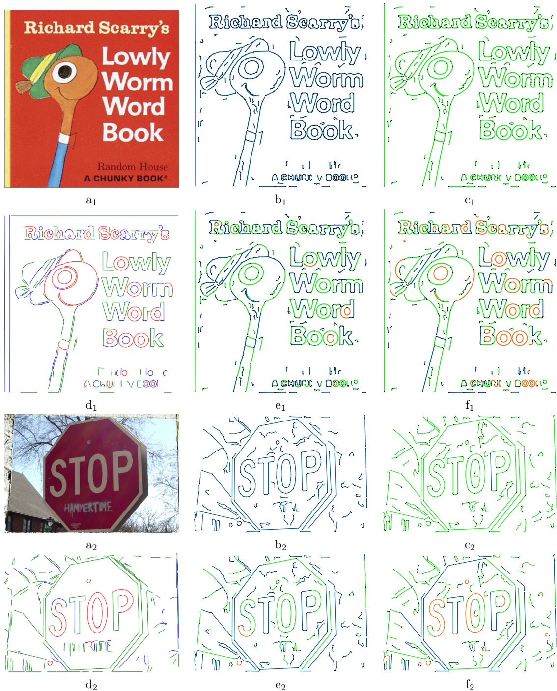
Figure 3.4: Comparison of the effect of pre-segmentation to the final result of DLCE on natural images and comparison to the results of ELSD. a_* : Given images as used in (Patraucean et al., 2012). b_* : Pre-Segmentation using Douglas-Peucker. c_* : Pre-Segmentation using circlePeucker. e_* and f_* : Final segmentation using b_* and c_* , respectively. d_* results of ELSD. Colours see Figure 3.2. We provide parameter setting and number of segments in Table D.2, page 189.
