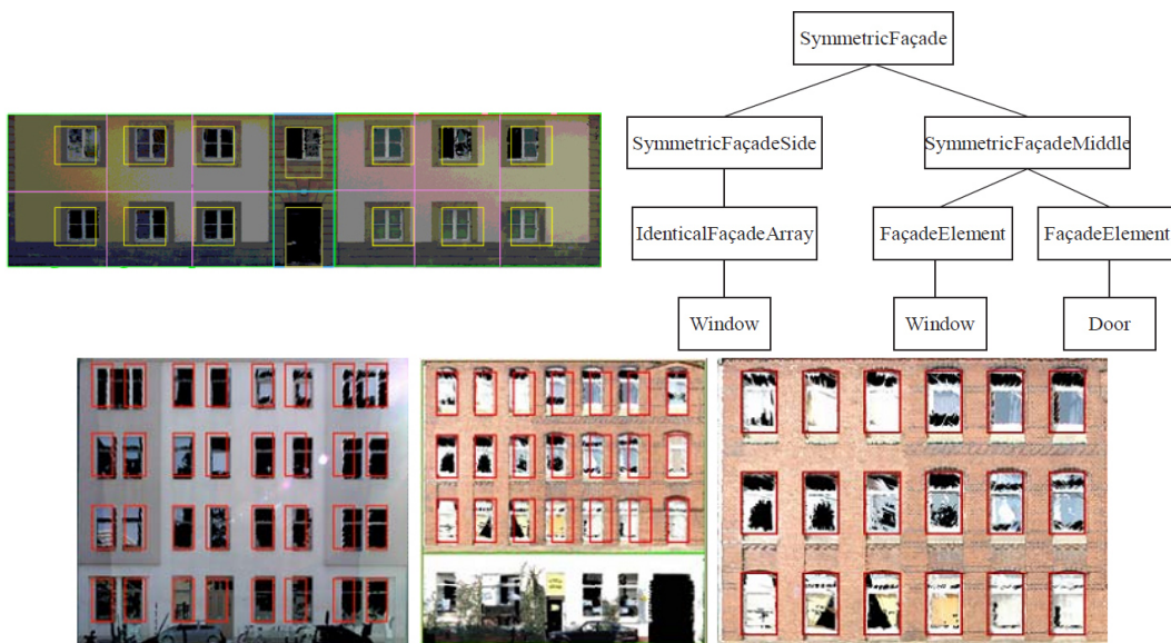
Figure 1.21: Grammar based facade interpretation. Top: Semantic partitioning of a facade and the according derivation tree, as shown in Brenner and Ripperda (2006) . Bottom: reconstruction results, as shown in Ripperda (2008)
