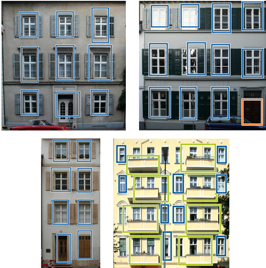
Figure 5.3: Results of object detection using the sliding window approach. We yield a reasonable detection rate, but accuracy of detected objects is low. Colours: blue - window, orange - entrance, green - balcony.
