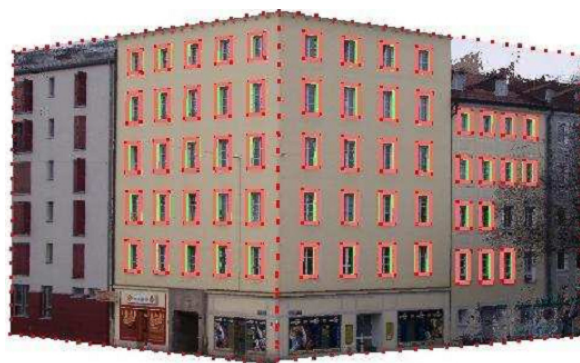
Figure 1.9: Result of window detection and 3D reconstruction, as shown in Reznik and Mayer (2008) . Found window hypotheses are marked as red boxes.
