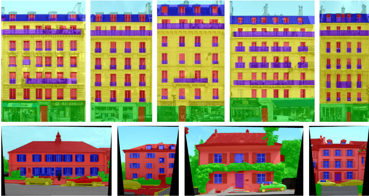
Figure 1.13: Results of facade image segmentation, as shown in Martinović et al. (2012) . They show results on complete building images, and furthermore, on facades showing less structure.
