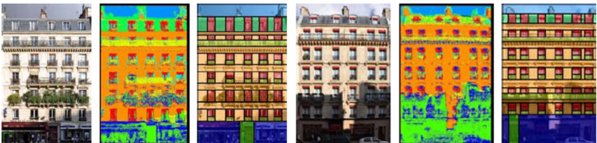
Figure 1.12: Facade image segmentation on Haussmannian buildings, as shown in Teboul et al. (2010) . Columns 1 and 4: original images. Columns 2 and 5: pixelwise classification. Columns 3 and 6: segmentation with procedural shape prior.
