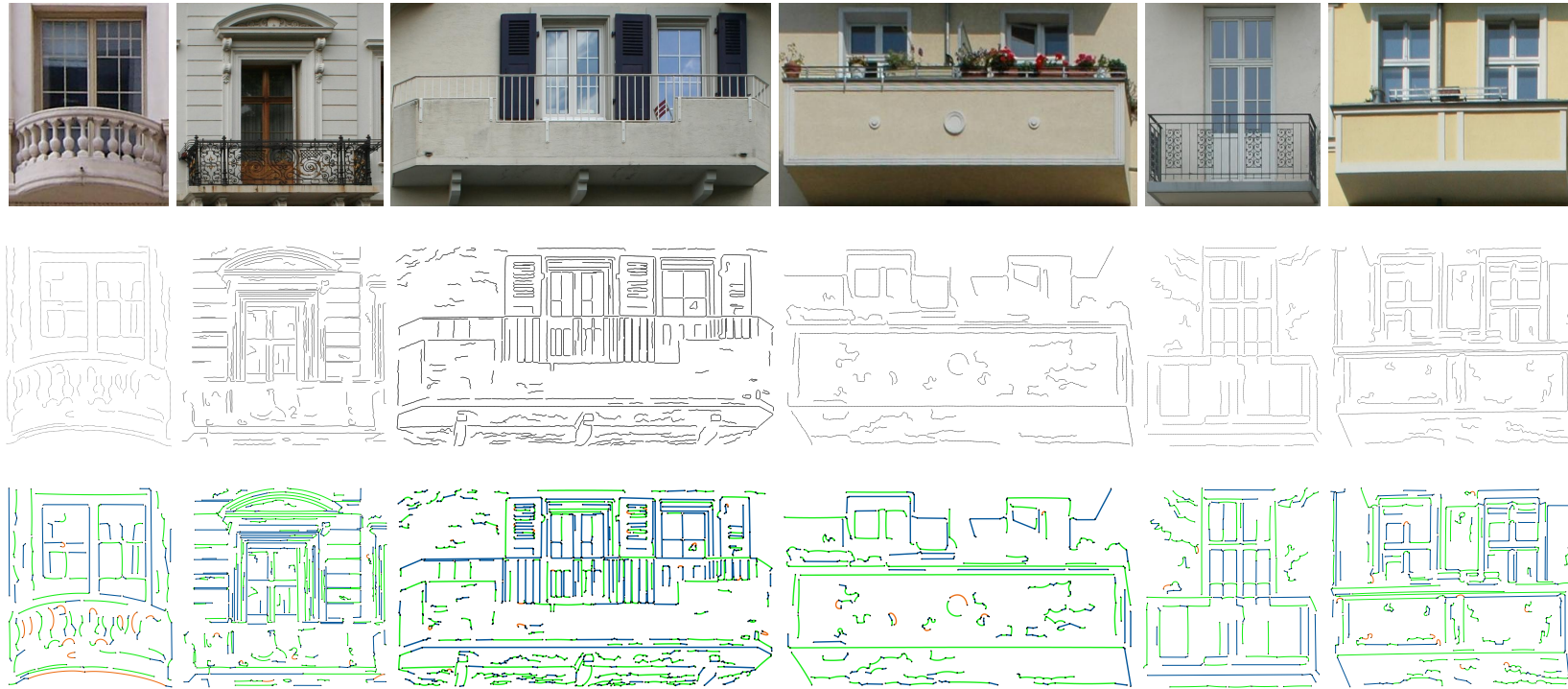
Figure D.3: Balconies. Results of DLCE on facade objects. Top row: Image patches. Middle: Extracted pixel-chains. Bottom: Results of DLCE. Colours, see Figure D.1.
