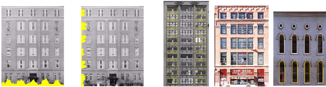
Figure 1.2: Window detection and reconstruction from single view rectified images, as shown in Lee and Nevatia (2004) . Left: Gradient projection. Right: Results after grouping similar elements and adding depth by plane sweep.
