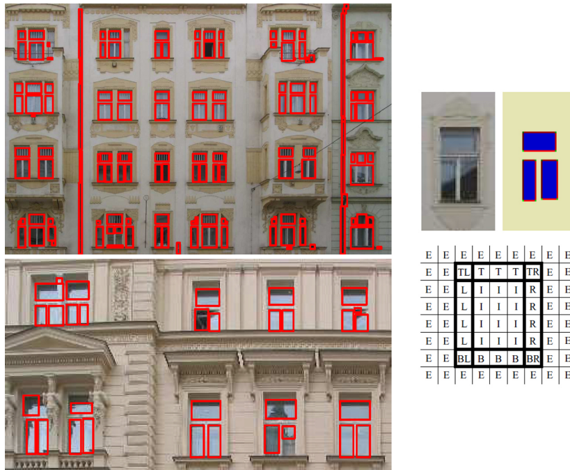
Figure 1.6: Results of window pane detection, as shown in Čech and Šára (2008). Left: detected window panes. Right: labelled image patch and allowed configuration of labels (E - external, I - internal windowpane label, (L,R,T,B) - (left, right, top, bottom edge), (TL, TR, BL, BR) - corners ).
