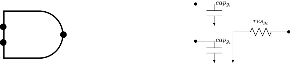
Figure 4.2: An AND gate and its switch-level RC circuit model: It contains a capacitance element cap_{g_i} for each input pin, and an output resistor res_{g_i} .
