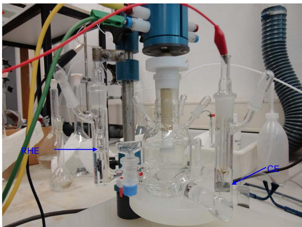
Fig. 2. Schematic and an actual photo of the experimental setup of RRDE with the glass cell containing the three-electrode arrangement.
