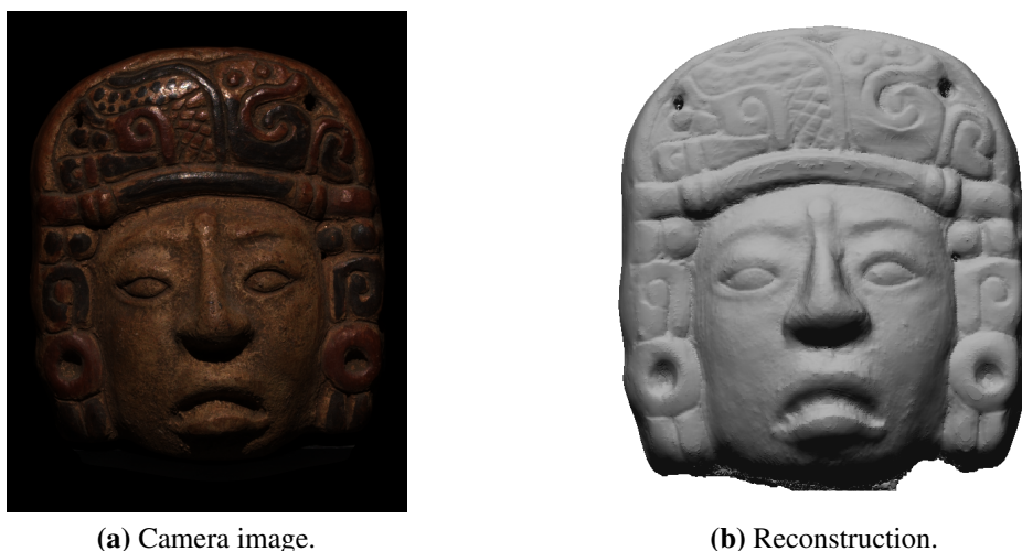
Figure 5.6: Results on a photometric stereo dataset: In particular, the painted regions of the clay mask exhibit specularities which leads to a violation of the assumption regarding Lambertian reflectance behavior. Nevertheless, the reconstruction preserves the shape in these regions. The robustness of our reconstruction technique originates from the outlier-robust normal estimation achieved by the mean-shift algorithm and a subsequent robust refinement step.
