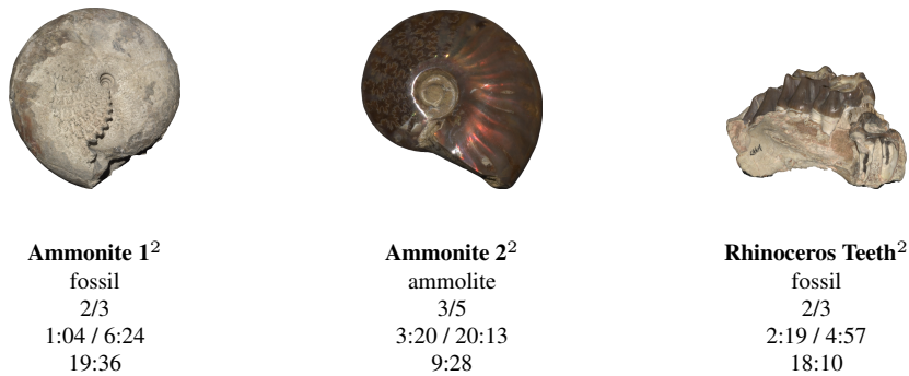
Figure 9.6: Objects digitized in the scope of [Sch14]: Listed are the respective apparent materials of the individual objects, the number of used exposures (geometry acquisition / reflectance acquisition), the acquisition times (geometry acquisition / reflectance acquisition) as well as the total processing times ( 1 Measured in the Dome 1 device, 2 Measured in the Dome 2 device, 3 Original measurement data damaged, 4 No information available due to data loss).
