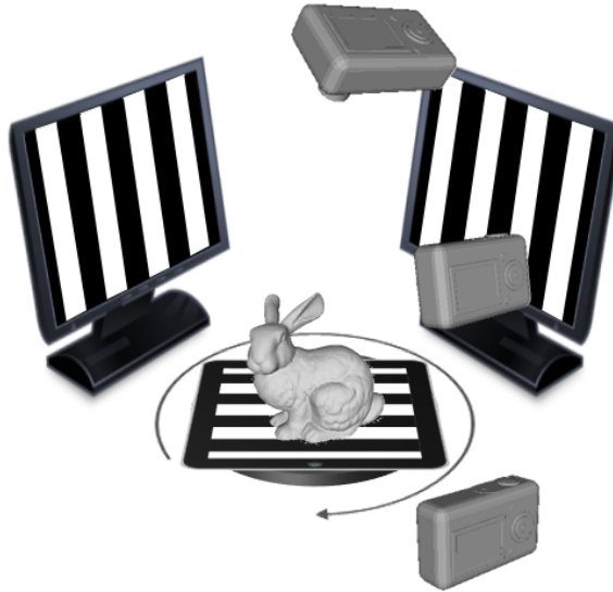
Figure 5.2: Sketch of the utilized setup: The screens successively display the series of patterns for each rotation of the turntable. The reflected pattern on the object surface is observed by the cameras. For illustration purposes, only three of the eleven employed cameras are drawn.
