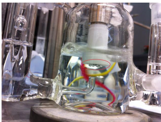
Fig. 3.8 Image of the formation of oxygen bubbles on 800\ \mu\text{g cm}^{-2} \text{Co}_3\text{O}_4/\text{Ag} electrode in the case of holding the potential at 1.8 V for 3 min in \text{O}_2 -saturated 0.1 M LiOH solution with a rotation rate of 10 Hz.
