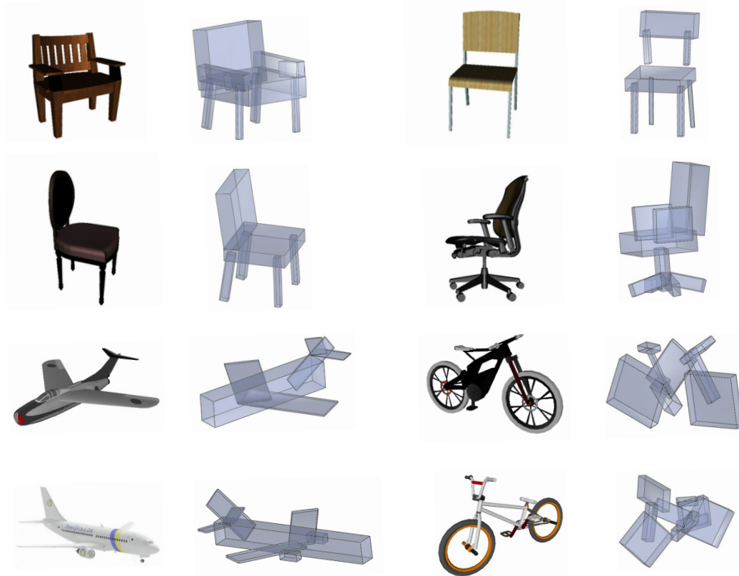
Figure 5.3: The left is the input RGB images, and the right is the inferred 3D shape structures by our VGG-RvNN autoencoder.
