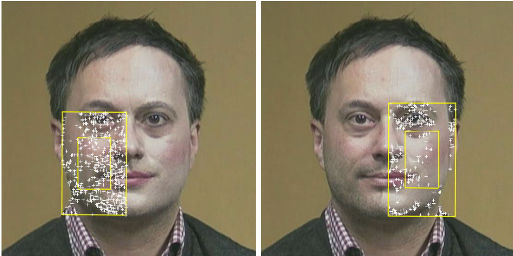
Figure 4.18: ROIs (with tracking markers) used for the makeup influence test. Left: Without makeup applied Right: With makeup applied
