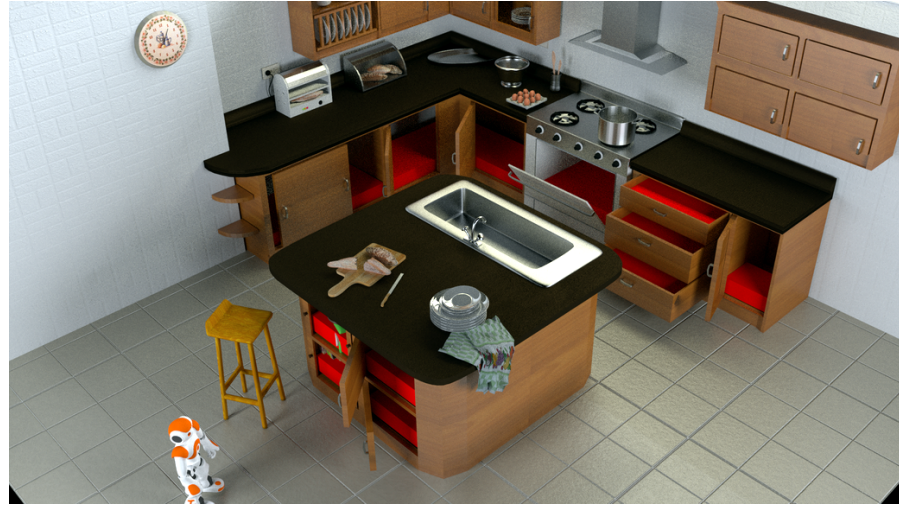
Figure 6.1: Nao inspecting a kitchen environment. The robot’s task is to search for an object in the user-defined regions of interest marked in red. Kitchen model based on [60].
