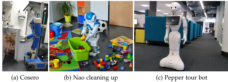
Figure 1.1: Robots acting in human environments. (a): University of Bonn’s Cosero opening a fridge to investigate its contents (source: [169]). (b): Our Nao robot cleaning up a children’s room as part of the SQUIRREL project (source: [158]). (c): Pepper robot providing an interactive tour of a lab at Queensland University (source: [166]).
