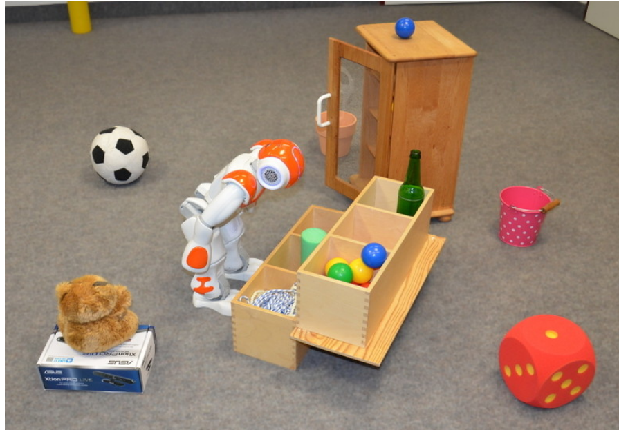
Figure 5.1: Nao inspecting an environment. The robot bends over to peek into a box for completing the task of completely covering the environment with its camera, e.g., for finding objects.
