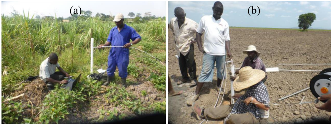
Fig. 3.4. Piezometer installation, (a), inland valley in Uganda, (b), floodplain in Tanzania.
