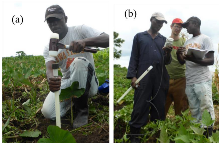
Fig. 3.6. Soil moisture measurement. (a), installation of soil moisture PR2 access tube; (b) reading soil moisture content using HH2 meter connected to PR2 sensor.
