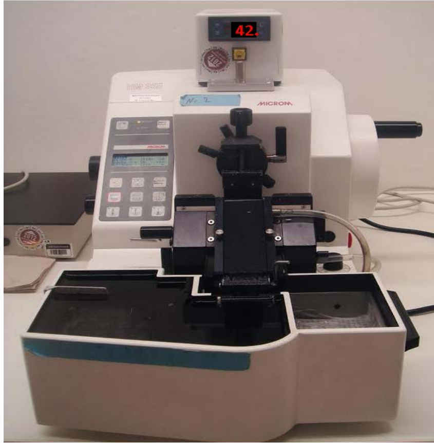
Fig. 25: A microtome, installed with water bath and heat sensor.
