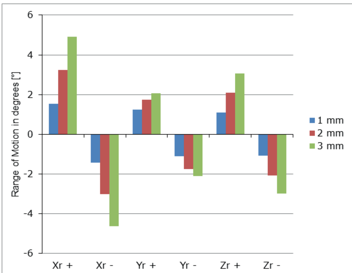
Figure 2: Graph of ROM in the modeled motion segment depending on the length of the IVD.
