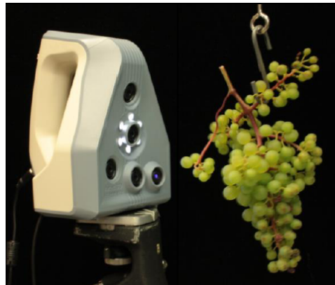
Figure 2.2: During the scanning process, the Artec 3D Spider Scanner (Artec 3D, 2019a) is placed in front of a grape bunch that is attached to a rotating hook. The grape bunch is scanned for slightly more than a full rotation period, generating a pointcloud that shows the grape bunch from all sides.
