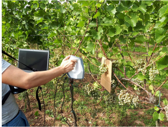
Figure 6.1: In the field, the grape bunch is scanned from the front, with a cardboard attached behind it as artificial, easy-to-remove background.
