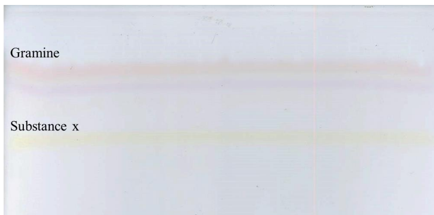
Figure 39: TLC separation of an organic extract from an Arthrobacter sp. GB1 culture treated with gramine.
