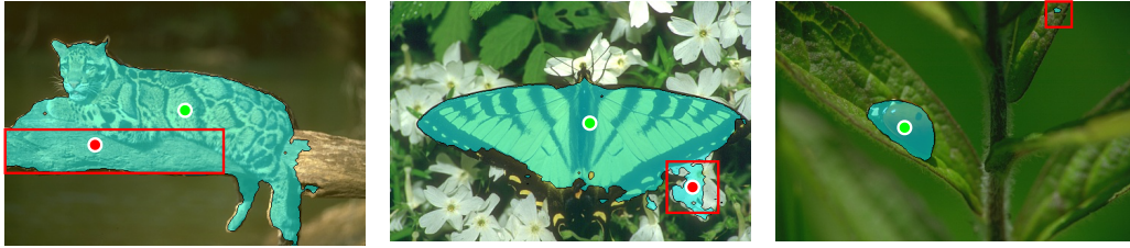
Figure 1.5: Segmentation masks generated from the networks are not always perfect. Given an initial positive click from the user (shown in green) on the object of interest, the generated segmentation masks (overlaid) shows false positive regions where the background pixels were marked as foreground. Here, the false positive error in the left image is significantly larger compared to the other images. We provide a rough visual estimate using the red bounding boxes. In order to refine the mask and remove the false positives, most interactive frameworks require the user to place a click in the center of the largest erroneous region (skipped for the right for ease of visualization). The corresponding refinement click is shown using a red circle. We note that these refinement clicks do not account for the spatial extent of the error which can vary to a large extent across different instances.
