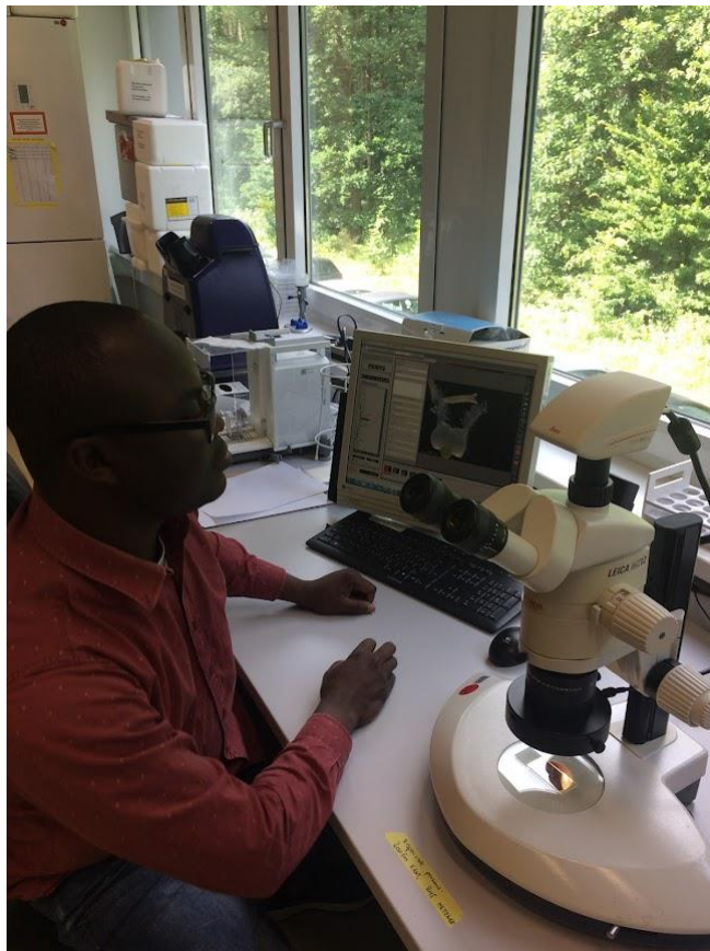
Figure 2.7 Author using the stereomicroscope (Leica MZ12 stereo microscope, Germany) to take barley floret images. The microscope is equipped with a built-in camera to capture images which are saved to a computer.
