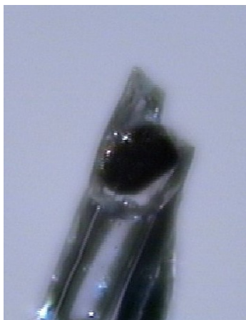
Figure 4.14: Black crystal of [\text{Eu}(\text{NH}_3)_8]_2[\text{Eu}(\text{NH}_3)_3(\text{As}_7)_2] mounted on a glass capillary. Crystal dimensions are 0.130 \times 0.084 \times 0.026 \text{ mm}^3 .
