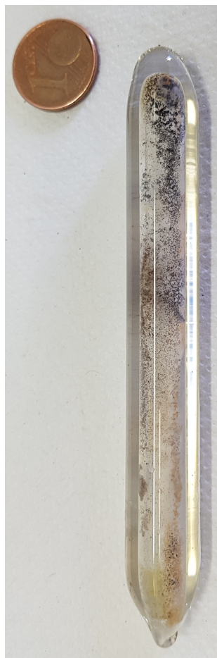
Figure 4.20: Black rod-shaped crystals of the new compound \text{Rb}_2\text{AuAs}_7 inside the reaction ampoule.
