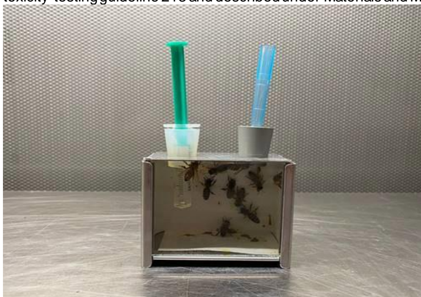
Figure S2. Honey bee cage used to feed worker bees according to OECD oral acute toxicity testing guideline 213 and described under Materials and Methods.
