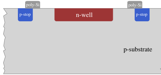
Figure 4.8: Simplified cross-section of an n-in-p pixel of the large-area passive CMOS sensor. Each pixel consists of an n-implantation (n-well) as the charge collecting electrode embedded into the p-type substrate. Small p-implantations (p-stop) isolate the pixels from each other. A low-resistive poly-silicon layer encloses the readout electrode. Metal layers are omitted.
