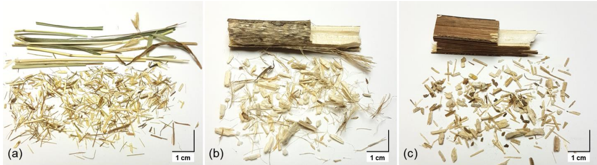
Fig. B 1: Blades of meadow hay (a) along with shoots of Virginia mallow (b), and cup plant (c) before and after grinding by the hammer mill (screen size 6 mm, round hole) used in this study. With a size scale of 1 cm.
