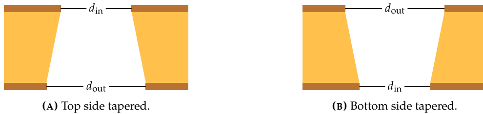
FIGURE 5.11: The profile of holes in a single conical GEM foil. Since the holes are not symmetric, there are two configurations. The tapered side can be on the top (A) or on the bottom (B).
