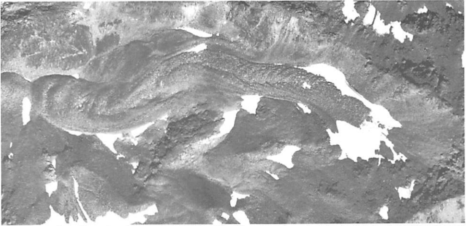
Underlying orthophoto of 20.08.1993 (flight-line 16, aerial photographs taken by Swisstopo). Plait-like ridge and furrow topography in the upper part of the rockglacier seems to result from sediment input of two different source areas.
