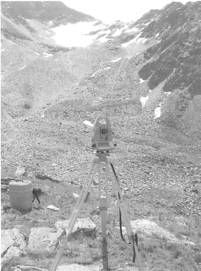
Fig. 3.7 Total-station on one of the reference points situated on a latepleistocene moraine with an overview of the research object (rockglacier in the background).
