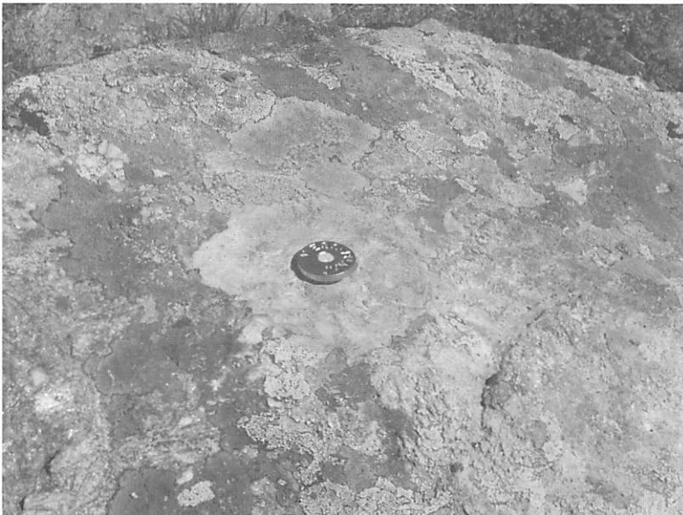
The thread, where the prism can directly be screwed into for the measurement, is protected by a plastic screw throughout the year.
