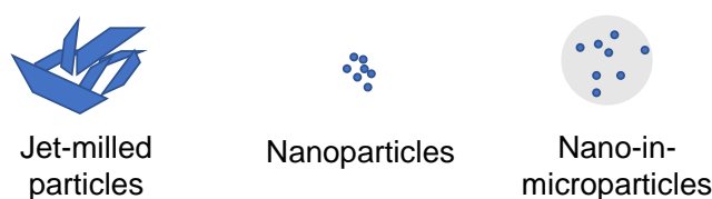
Figure 1: Schematic illustration of examples of (engineered) dry powder particles. ■ API, ■ matrix former
