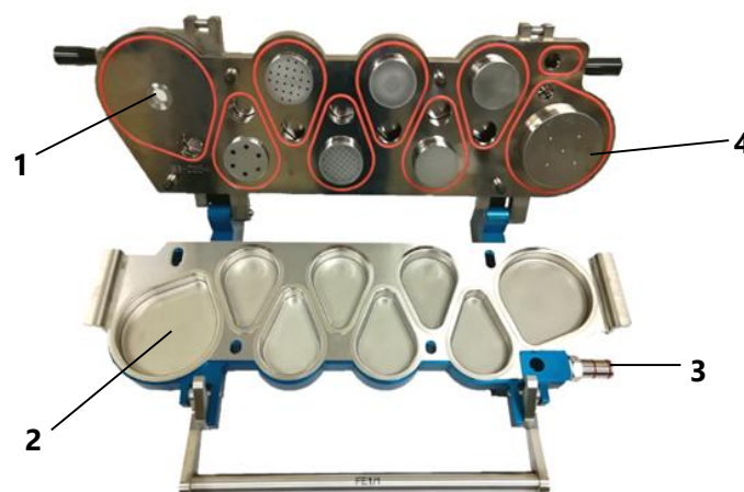
Figure 11: NGI (Apparatus E) for the assessment of fine particles according to the Ph. Eur [80]. The lid consists of a steel body with nozzles of a defined number and diameter (e.g., Stage 1 nozzle (1) or micro-orifice collector (MOC) (4)) and interstage pathways. The bottom frame comprises a tray with removable impaction cups (e.g., 2) and a connection to the vacuum pump (3). © Boehringer Ingelheim
