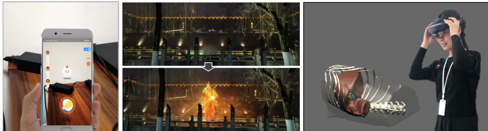
Figure 1.1: Three different ways for visualize augmented reality information. Left: show virtual model on screen of smart phone. Mid: visualize virtual information with 3D projector. Right: show virtual information with OST-HMD.
