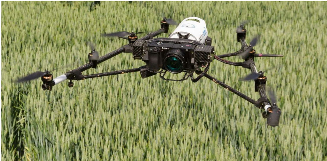
Figure 4 Falcon 8 octocopter used for data acquisition in the presented study (image provided by Ralf-Uwe Limbach).
