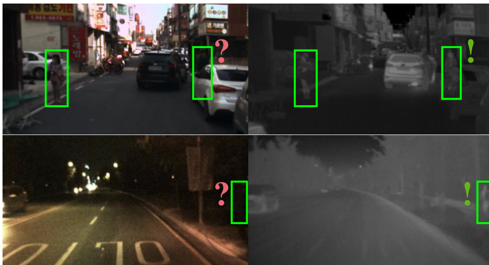
(c) For two scenes we show the visible image on the left side and the corresponding thermal image on the right side. Thermal cameras measure the long-wavelength infrared radiation. They are therefore well suited for detecting pedestrians at night or in low lighting conditions. Although the pedestrians are poorly illuminated in both scenes, their appearance can be clearly perceived in the thermal image.
