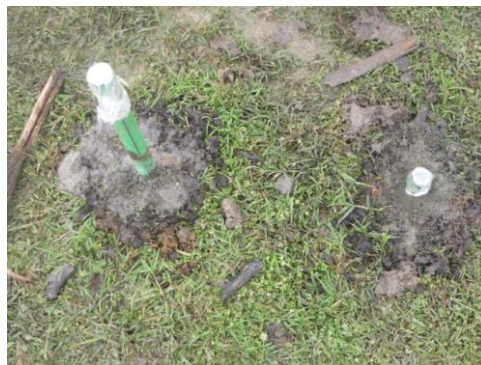
Fig. 4.3: Piezometers installed in the field.
