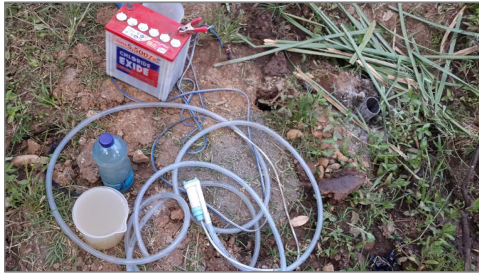
Fig. 4.5: Sampling of groundwater from wells and piezometers with a hand pump linked with a battery.
