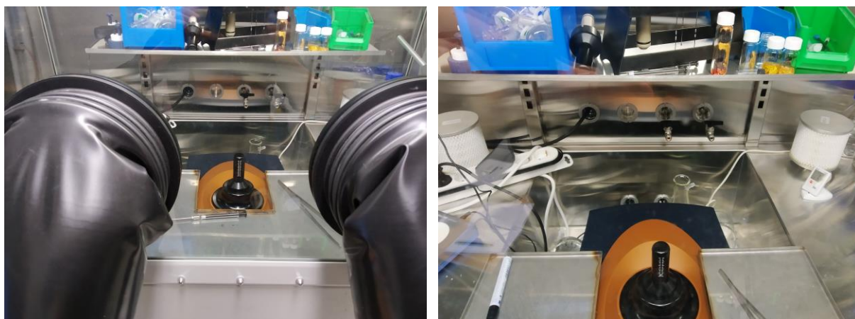
Figure 5.10. System of IT-Calorimeter of AK Schneider inside the glovebox. TA Instruments NanoITC equipped with a 24 K gold cell with a sample volume of 1 mL operated in overfill mode and controlled by the ITCRun software version 3.4.6.0.
