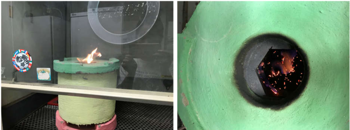
Figure B.1 Production of biochar.
