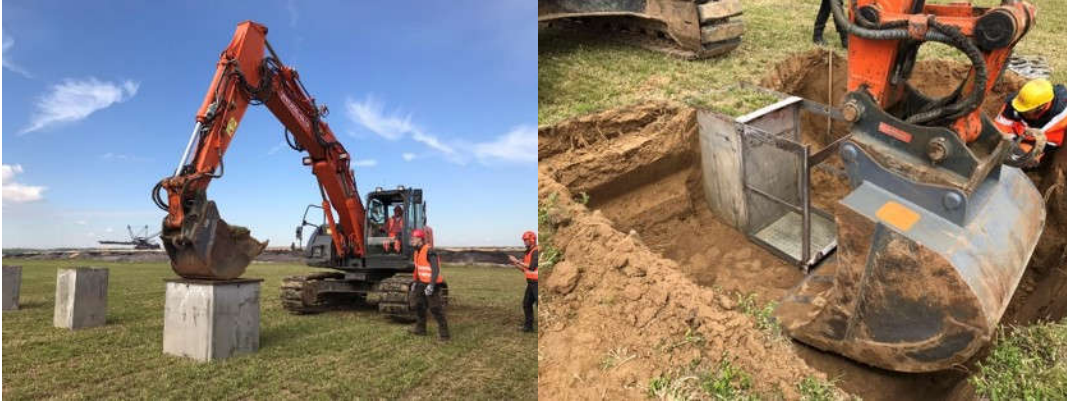
Figure 1.4 Sampling of the soil monoliths for the lysimeter experiment.
