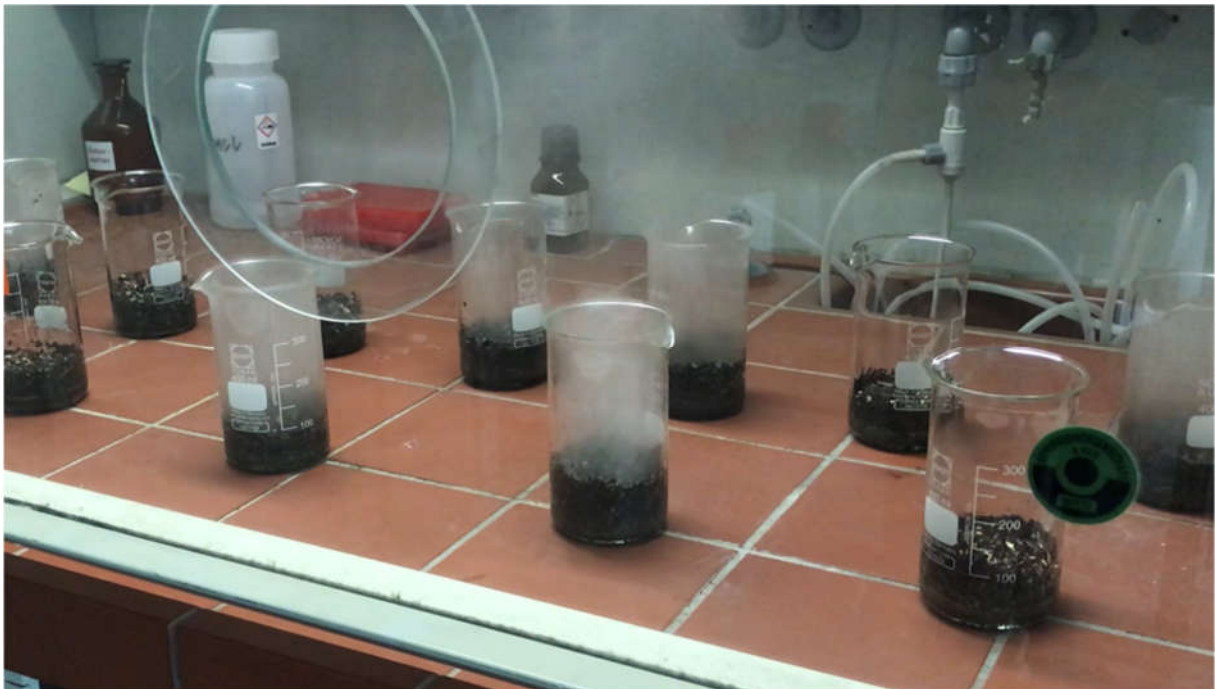
Figure B.2 Oxidation of biochar.
