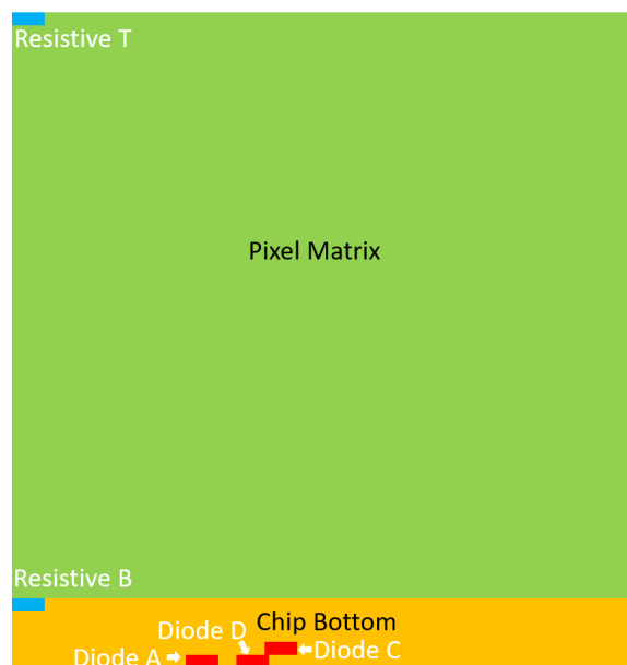
Figure 6.4: Location of the five RD53B temperature sensors.
