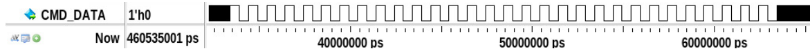
Figure 5.1: Slow clock command applied to the command input of RD53B for initial reset.
