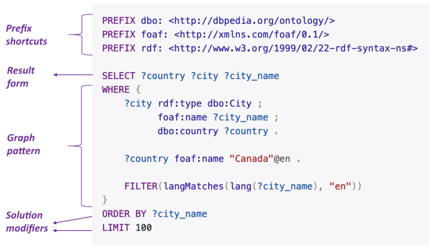
Figure 2.6: An illustration of SPARQL query components.
