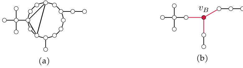
Figure 2.1: (a) Outerplanar graph with face number 4 and (b) its corresponding block and bridge tree. The vertex v_b (in red) is the newly created block vertex connected by the red edges to the rest of the block and bridge tree.
