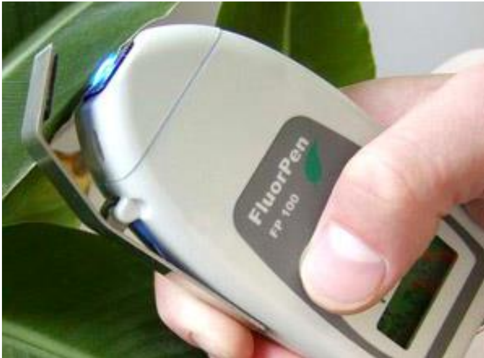
Figure 9. FluorPen is a portable, battery-powered fluorometer that enables quick and precise measurement of chlorophyll fluorescence parameters in the laboratory, greenhouse, or field. It can be effectively used for studying photosynthetic activity, stress detection, herbicide testing, or mutant screening (Photon Systems Instruments, 2016).
