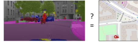
Figure 1.6: P4) Geo-Informed Validation. We use Informed ML to validate autonomous driving models with prior knowledge from street maps. For example, the left image shows a segmentation of a traffic scene in the Cityscapes dataset [15] and the right image shows the corresponding map [43]. Here, a road intersection to the right is not detected in the segmentation, but is given by the map. Such potential errors of AI modules can be identified with Informed ML.
