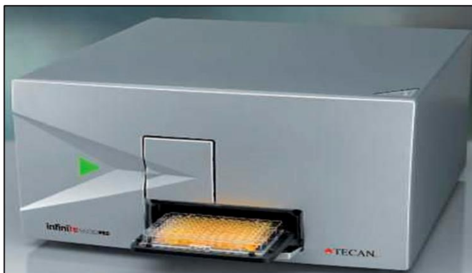
Figure 4.3: Tecan Infinite 200 PRO microplate reader for absorbance measurement
