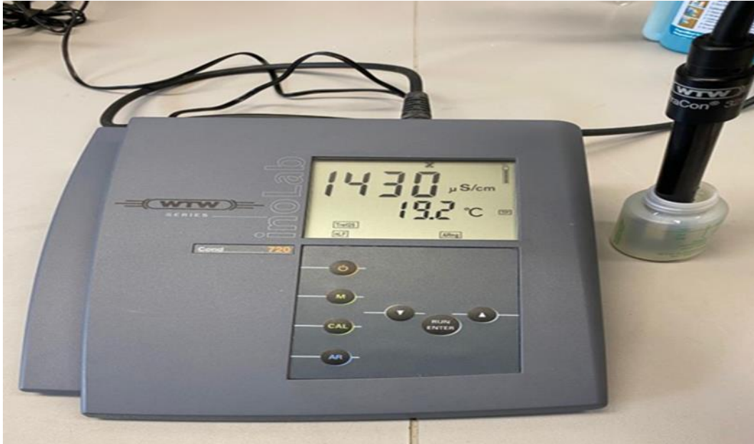
Figure 4.1: WTW inoLab PH/Con device used to measure electrical conductivity
